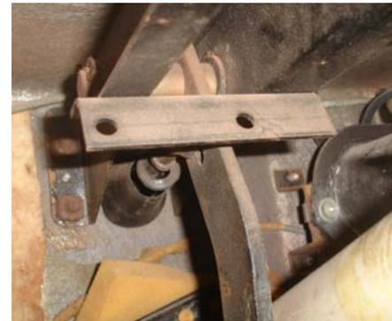
scrap piece of steel to make a bracket for the switch, measuring, marking and drilling the proper holes with my drill press (though a regular drill will work just fine if you clamp the work piece in a vice.)
