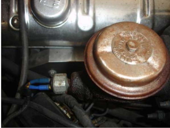
As mine was not working, I decided to change it over to a mechanical switch that mirrors what is used on nearly all modern cars. There are advantages to this change. First, the brake lights now activate instantly when the pedal is moved, unlike the old system where the pedal has to generate full pressure to activate the switch and light the lamps. Second, the old style switch is troublesome and a potential point of hydraulic failure as it actually taps into the brake hydraulics.
